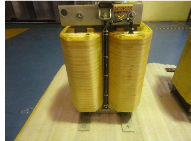
Inductor for Wind Power 730 A, 0.3 mH
