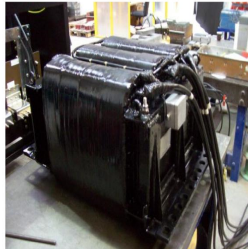
3-phase Auxiliary Transformer (320kVA, 800kg)
