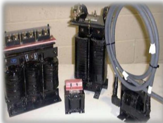
Battery Charger Components (90kW, total 255kg)
