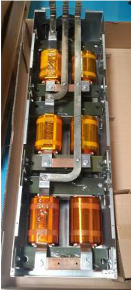
LC Assy for Solar Power Application Inductor Assembly- 420A, 0.146mH
